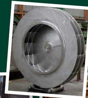
Repair and manufacture of fan runners.
