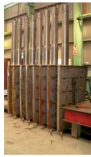
Rudders for Royal New Zealand Navy Project Protector vessels.
