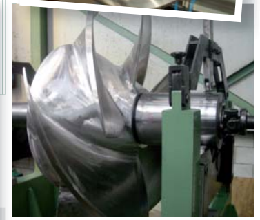
Impellor and wear ring for 80 cubic metre per second water jet propulsion unit.
