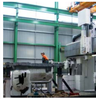
Steam turbine casing in 5 face double column machining centre.
