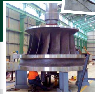
Overhaul of Large Francis Runners
