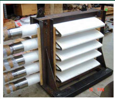
Refurbishment of Guide Vanes (Wicket Gates)
